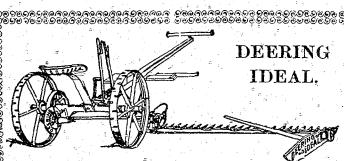
Deering Ideal Mower with Roller and Ball Bearings, \$ serrated ledger plates, adjustable drag bar and shear cutting knives. The only mower that can be drawn at a slow walk or started in any crop without backing the
