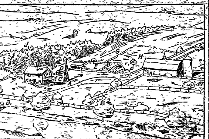
Illustrating Common But Unsafe Location of the Farm Well and Spring. Possible Source of Pure Water Also is Indicated. A, Unsafe Well; B, Unsafe Spring; C, Privy; D, Garden; E, Chicken Yard; F, Hog Yard; G, Cultivated Field; H, Pasture; J, Wooded Fenced Off and Kept Clean. Here, Beyond the Probable Channels of Impure Drainage, May Be Pure Water.
