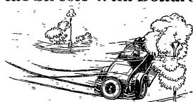
On any hard surface roadway, you frequently see black streaks, the result of unequalized brakes. When such brakes are applied one or more wheels lock, the rubber is ground off the tires, the car may skid and endanger lives.
