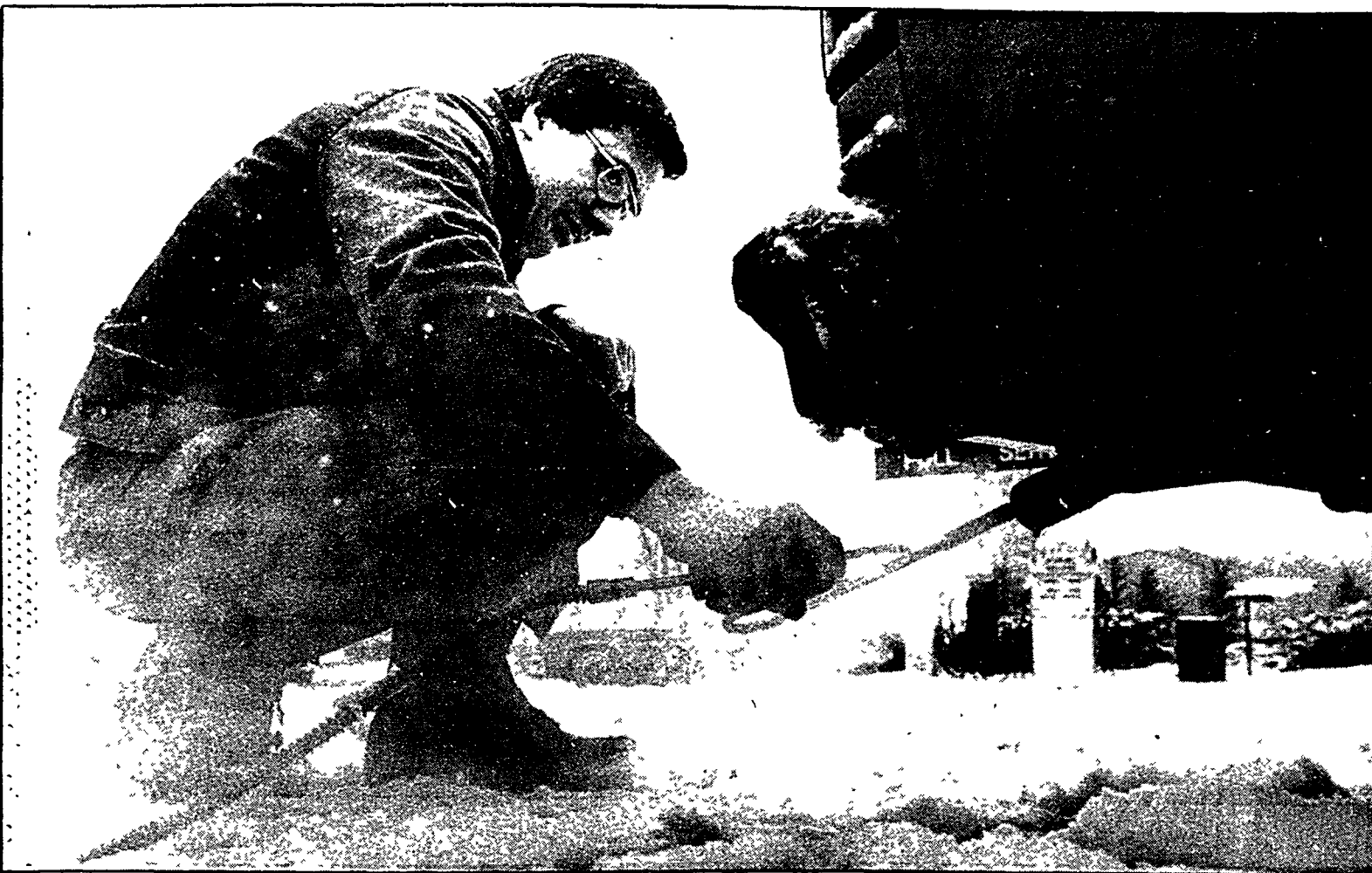
Jim Davis insets the probe into a car's tailpipe during exhaust test
