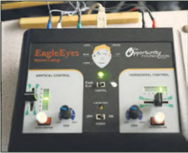
The EagleEyes' controller box that is wired to the sensors attached to students' faces.
