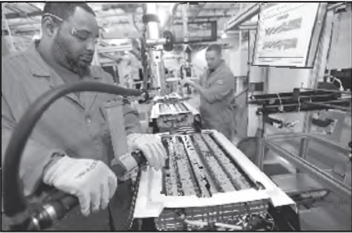
Battery packs for C-Max come together at Ford’s plant in Rawsonville.
