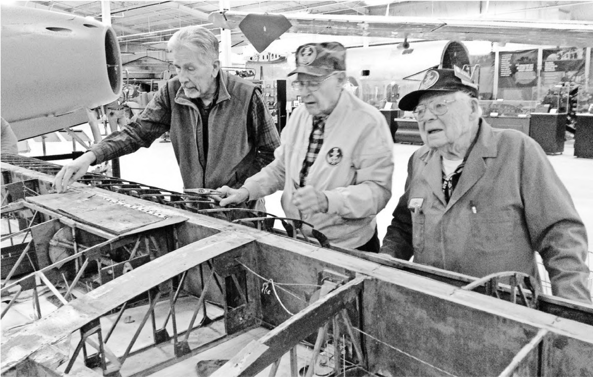
Restoration manager Ralph Koehler of Livonia (from left), Joe Kosek of Westland and Gene Blanchard of West Bloomfield look at how to remove a spoiler from the wing of a TG-3 glider that's being restored at the Yankee Air Museum.
