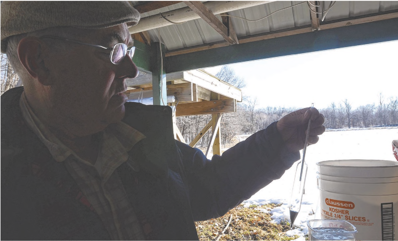
JOHN HEIDER | STAFF PHOTOGRAPHER John MacInnis checks the sugar content of the sap with a hydrometer. It's important to figure out how much sugar the sap has, as it will have differing boiling points.
