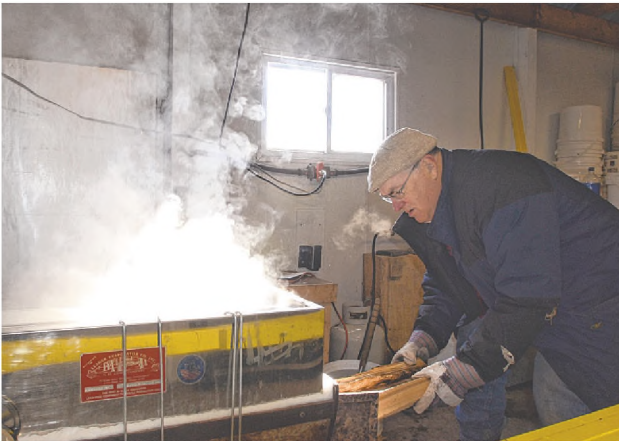
JOHN HEIDER | STAFF PHOTOGRAPHER Tollgate Farm volunteer John MacInnis adds a couple of logs to the sugar shack's boiler March 12. The boiler will reduce the amount of water in the sap to the point where it will finally become syrup.
