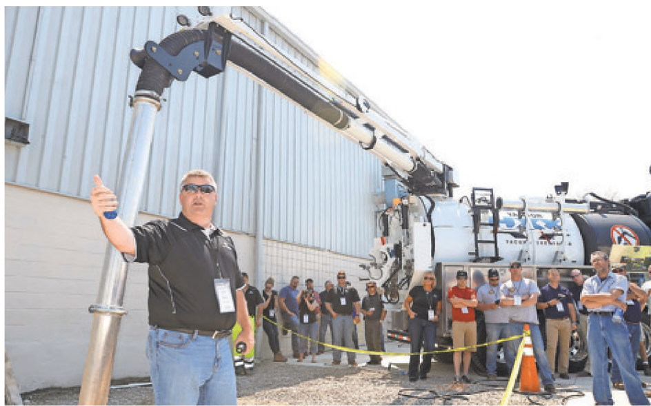
JOHN HEIDER | STAFF PHOTOGRAPHER Mike Suitor instructs industry representatives on how to use a Doheny vacuum truck for hydro-excavating during the Northville business' recent open house and seminar. Hundreds of workers from the U.S. and Canada stopped by to see the latest gear Doheny has at its Northville shop.
