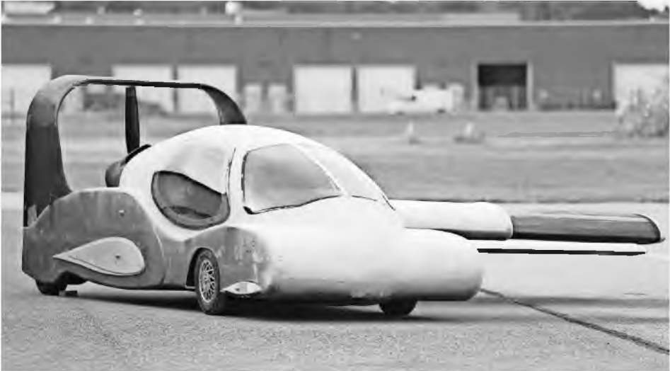
Sanjay Dhall’s flying car has airplane wings that telescope into the body so it can operate on roads.
