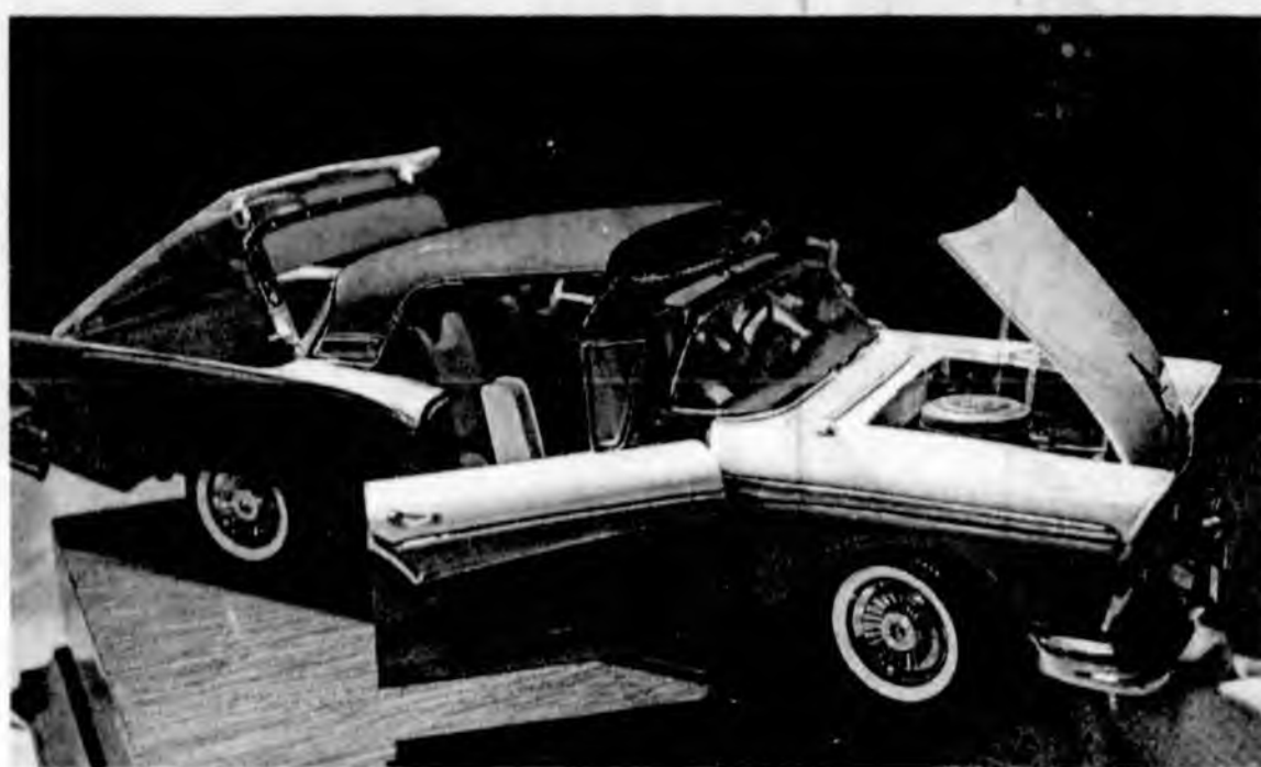
The 1950 were a hot time for American automobiles. The Ford Skyliner featured a retractable metal hard top. This model hints at the mechanical complexity of the design. BILL BRESLER | HOMETOWNLIFE.COM
