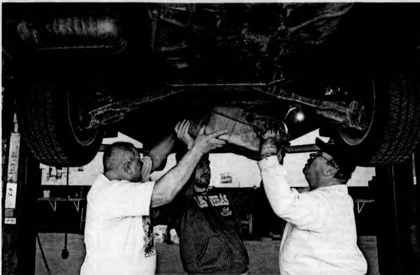
Under a lift, from left, Jerry Carson, his son Andrew, both of Canton, with their friend Dewie Smith of Northville, carefully drop the gas tank off Andrew's 2007 Ford Focus at My Mechanics Place in Livonia, Thursday, April 11, 2019. They have to remove the gas tank from the car in order to replace the fuel pump. JUNFU HAN, DETROIT FREE PRESS
