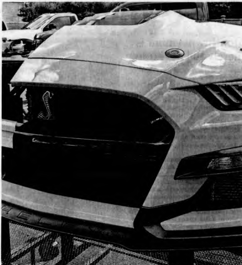
A bigger opening in the nose helps cool the GT500's 760-hp V8.
