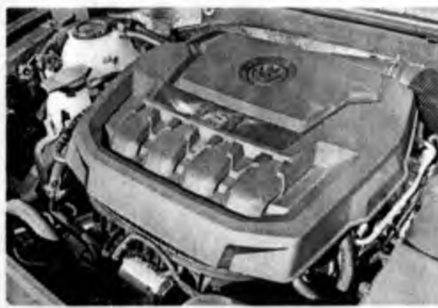
The Passat's 2.0L turbocharged engine produces 174 hp and 206 lb-ft of torque.
