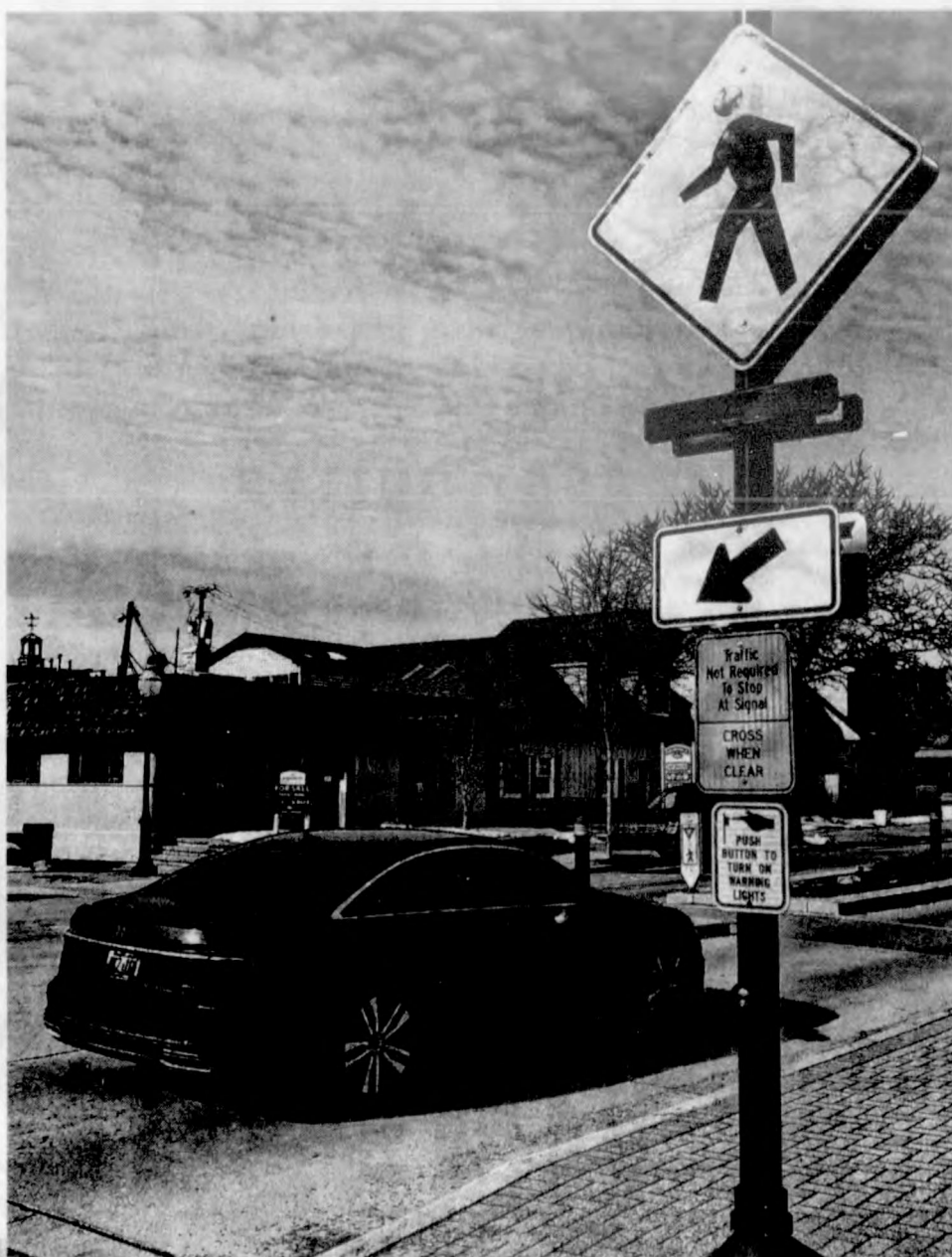
A Rectangular Rapid Flashing Beacon at Ann Arbor Trail and Forest in downtown Plymouth. The city installed several of the beacons around town in recent years, hoping to assist in pedestrian safety by alerting cars to someone looking to cross the road. DAVID VESELENAK/HOMETOWNLIFE.COM
